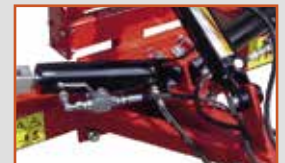
Two hydraulic cylinders with ball valves
