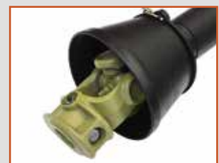
Driveline with shear pin safety
