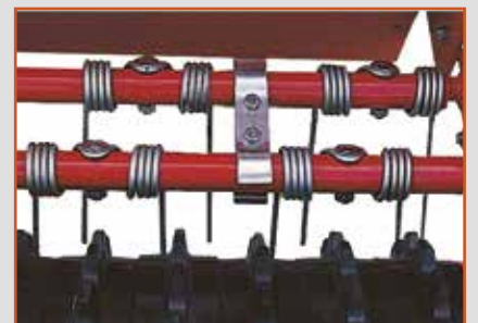
Tickler tines for partial or complete seed incorporation into the ground
