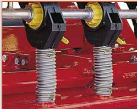
Precise seed metering cups
