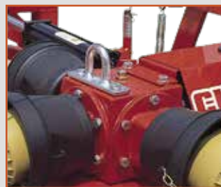
Heavy duty center-splitter gearbox
