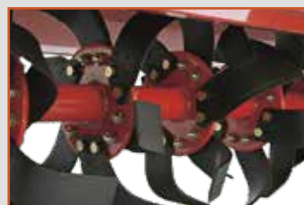
Rotor with 6 blades per flange
