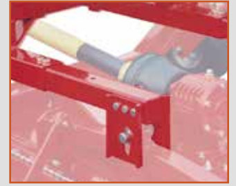
Telescopic wings that allow for adjustable cutting width to increase or decrease mower overlap
