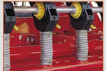
Precise seed metering cups
