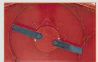
Rotor with free swinging blades
