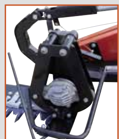
Cast aluminium connecting rods with cooling fins
