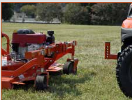
Front mount application with 2" receiver hitch
