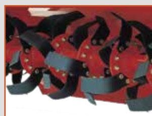
Rotor with 6 blades per flange
