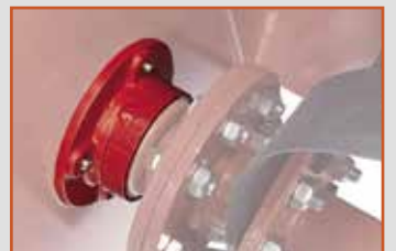
Stamped steel rotor shaft supports and transmission
