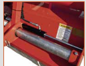
Hydraulic cylinder for side shift
