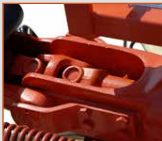
DRP-480 double yoke joint transmission
