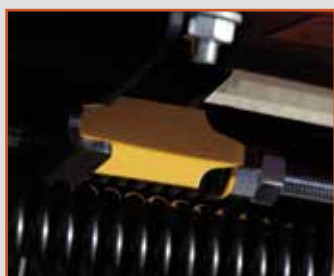
Easy to inspect and adjust belt tensioner
