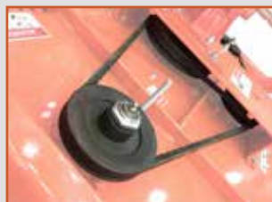
Two heavy duty reinforced belts (SPBX) with manual tensioner provide over 180° coverage of all pulleys and reduce belt maintenance
