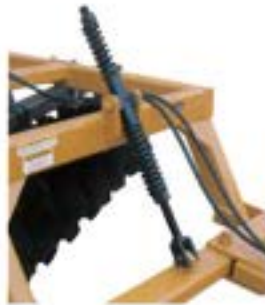
Front to rear leveling controlled by simple spring adjustment rod
