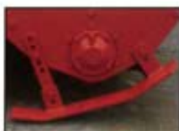
Tilling depth is controlled by adjustable skid shoes - to a maximum 8" depth.
