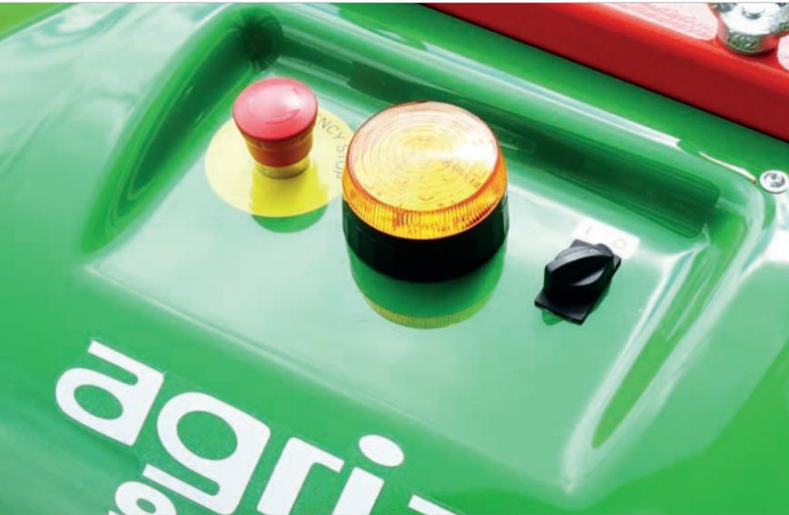
Both the machine itself and the remote control have an **emergency shut-off switch**, which stops the machine immediately when pressed.
