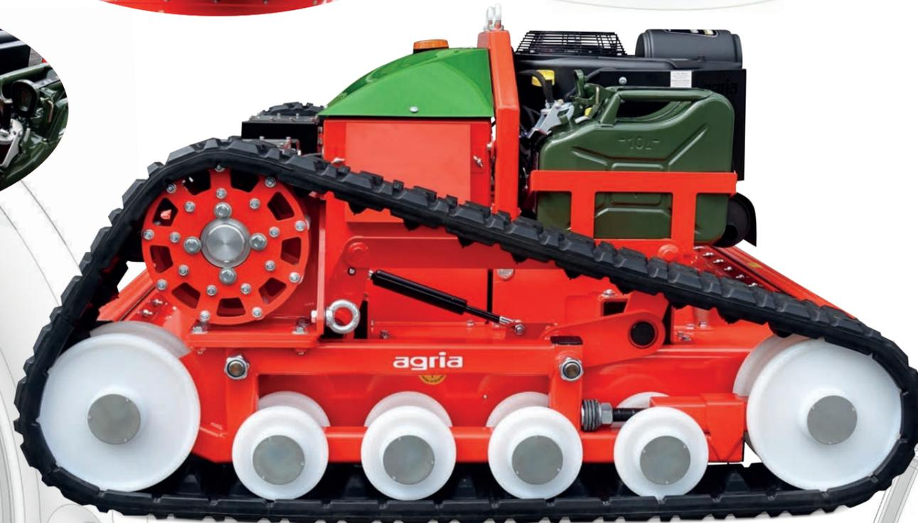
The two maintenance-free **reduction transmissions** transmit the power to the drive wheels
