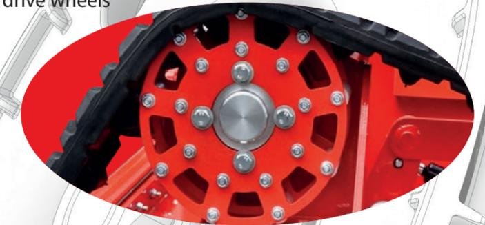
**Each drive** with a torque of more than 500 Nm
