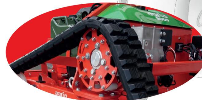
The electric hybrid drive is about **65% more efficient** than a fully hydraulic drive system.
