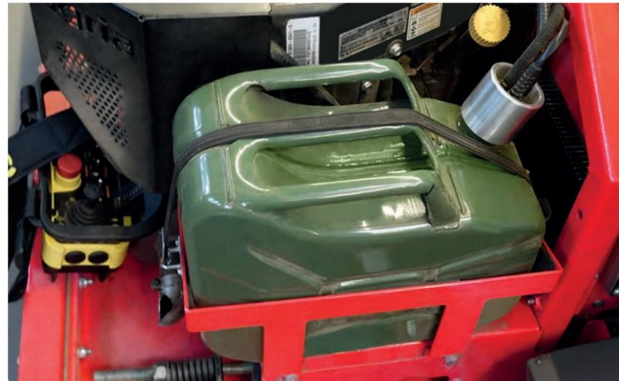
The **Replacement-fuel-canister-system by Agria** makes refuelling easy and safe even in difficult terrain. Two standard 10 liter canisters can be easily removed, replaced and reconnected. With this system, the agria 9600 can even be used in water protection areas without any problems.
