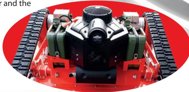
The **generator** generates electricity in Safety Extra Low Voltage (48 V)
