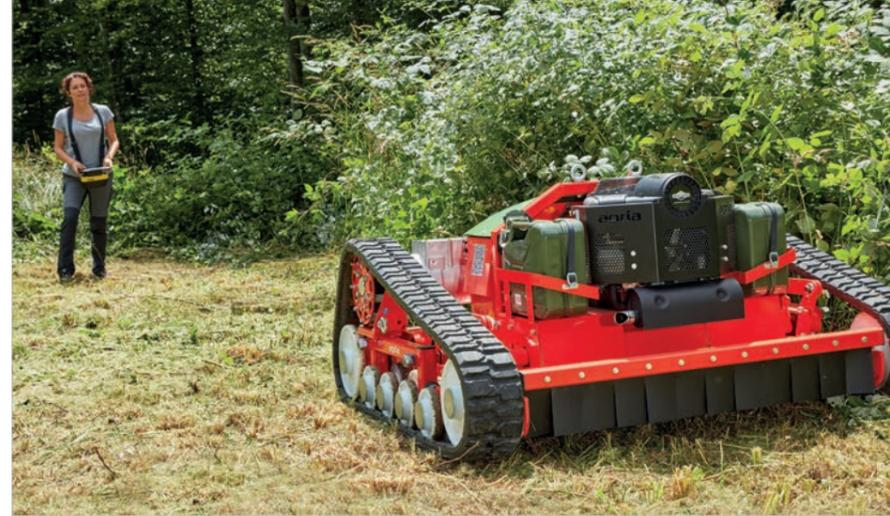
If a frequency is disturbed, the remote control **changes** to a **different frequency** in the frequency band **automatically**.
