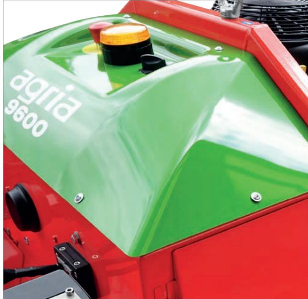
The entire electronics are placed in an easily accessible **electrical control box**. The E-box protects the components against dust and moisture, and because of the rubber buffers also against vibrations.
